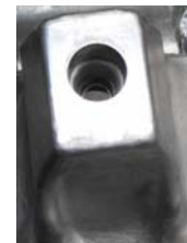
Figure 6. The precasted hole obtained by using the coated insert
