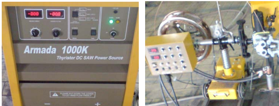
Fig. 1. SF welding equipment ARMADA 1000K: a) source; b) welding track
