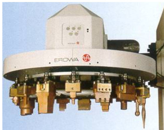
Fig.4. Horizontal rotary tool storage device EROWA.
