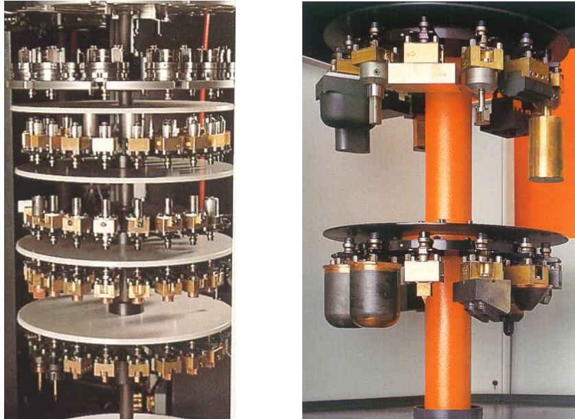
Fig.3. Vertical tool storage devices, for CNC machines.
