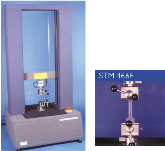
Fig.1 tensile testing machine SATRA (STM 466) with 466F attachment
