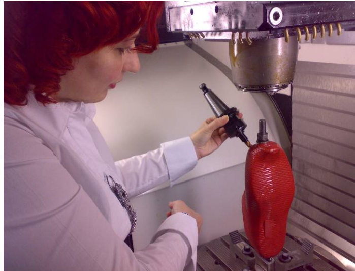
Figure 12 - Positioning of the last and finger-type cutter for processing
