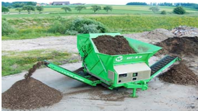
Fig. 4.1. Compost sorting plant
