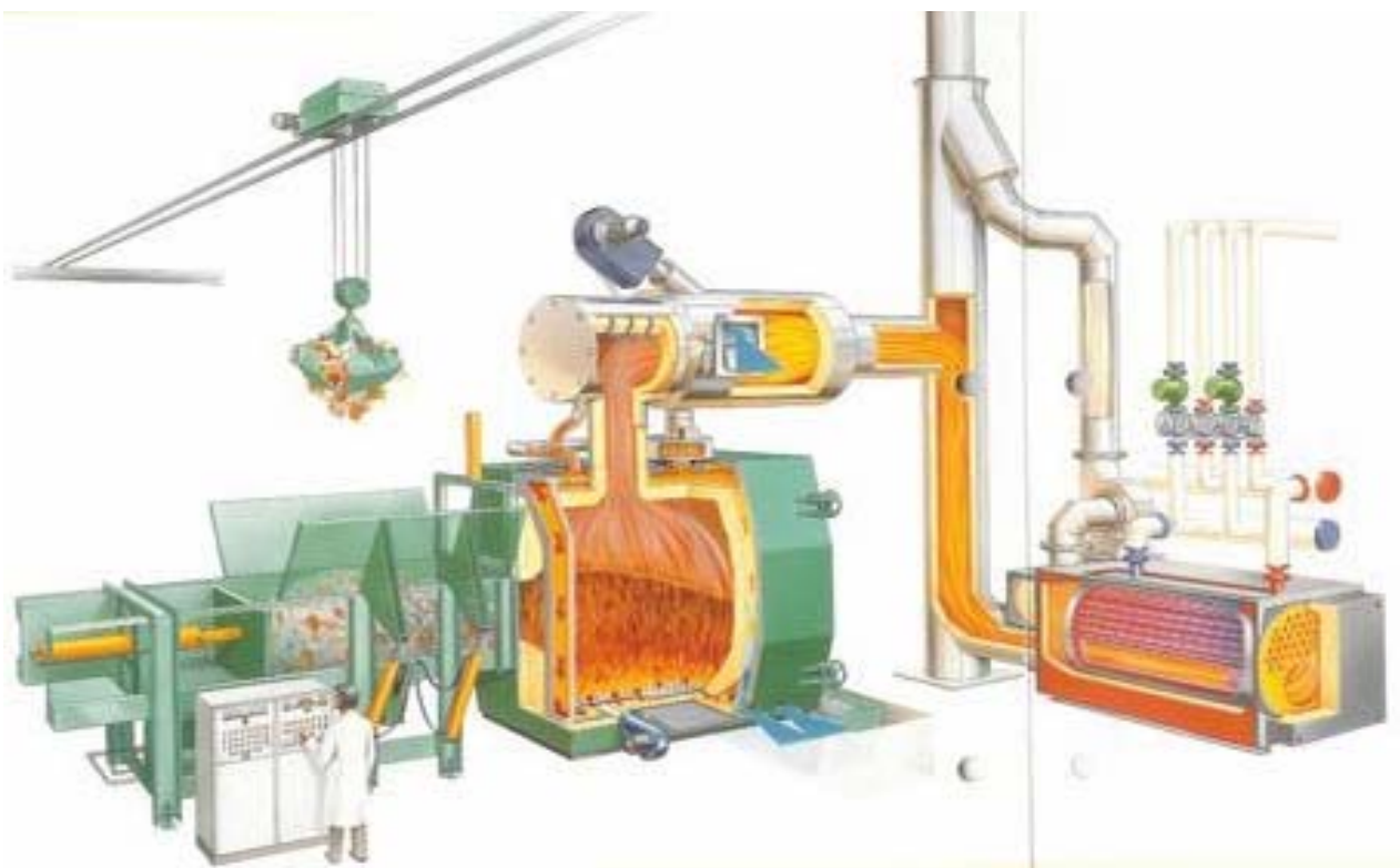
Fig. 3.1. Waste incineration installation type HOVAL MULTIZON
