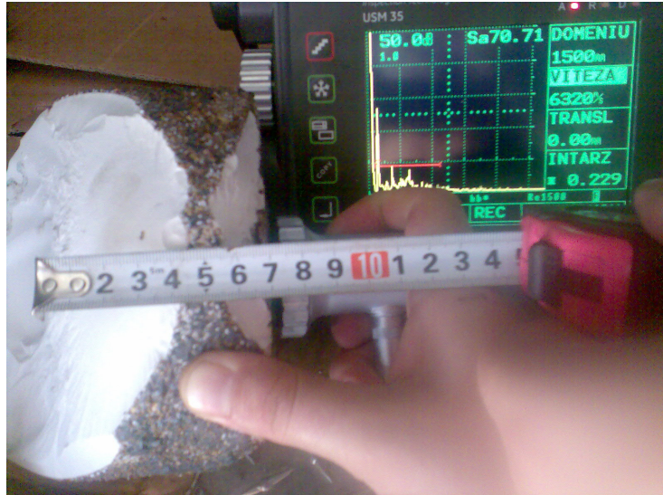
Fig. 2.5. Confirmation of the discontinuity indication at 70 mm.
