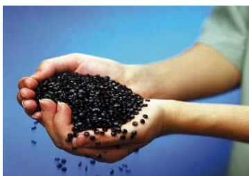
Figure 3: Raw material of PE in granules
