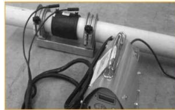
Figure 18 . Sleeve coupling ready for welding
