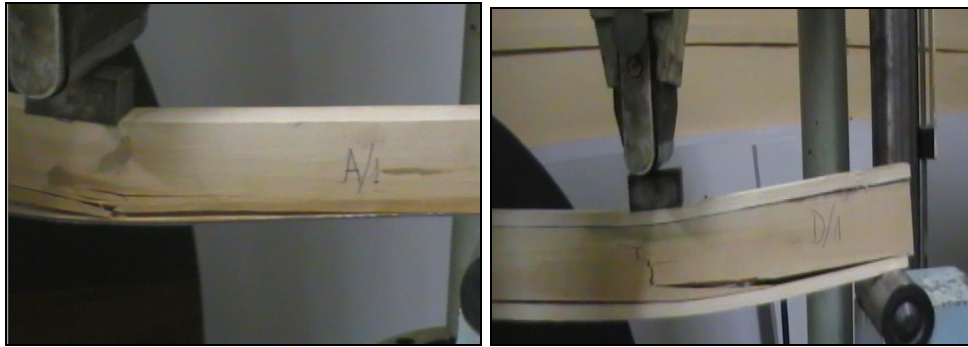
Fig.3 Bending test of laminated wood beams reinforced with: 1 plate CFRP (left) and 2 plates CFRP (right)
