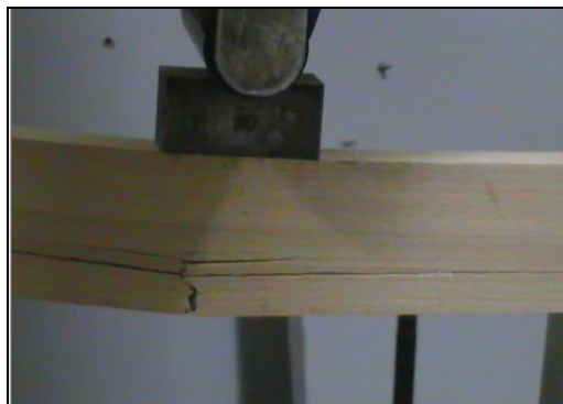
Fig. 2 Bending test of an un-reinforced wood beam
