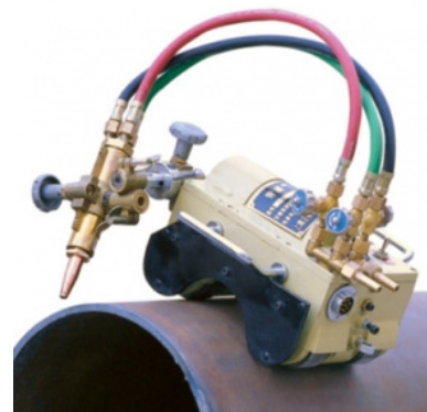
Fig.3. Tractor with magnetic fastening, cutting and welding.
