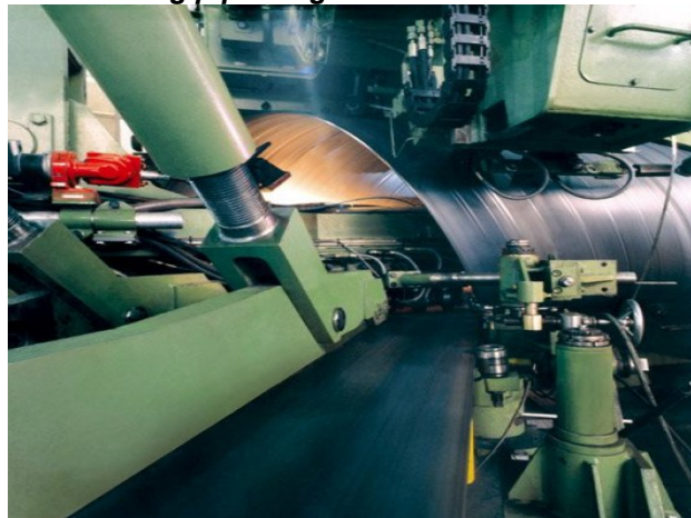
Fig.9. Manufacturing process for spiral welding
